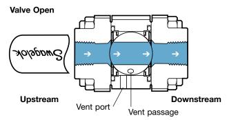
When the valve is closed, shutoff occurs only on the downstream side. Upstream fluids flow through the vent passage to the vent port and are released to atmosphere.
