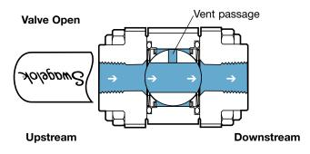
When the valve is closed, the vent passage faces downstream, allowing pressure to equalize between the body and the downstream system.
