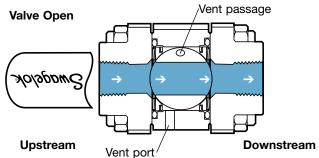
When the valve is closed, shutoff occurs only on the upstream side. Downstream fluids flow through the vent passage to the vent port and are released to atmosphere.
