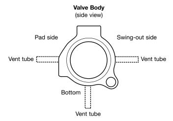
Tubes welded to vent ports allow controlled release or recovery of vented fluids.
