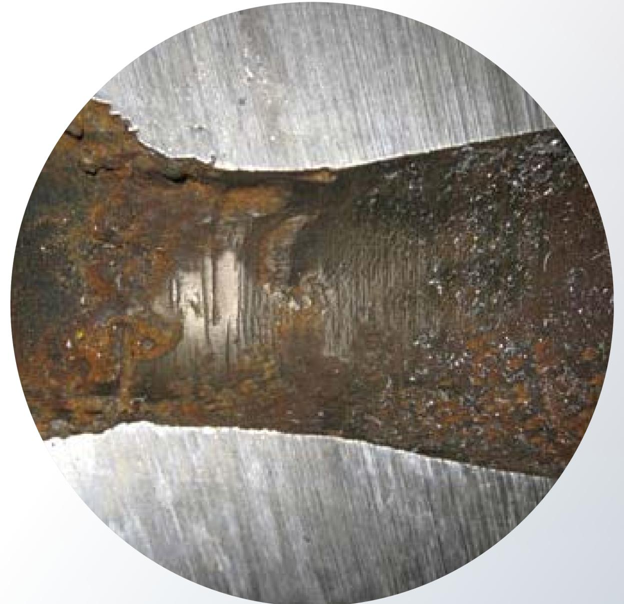
Reprinted from Science Direct, Volume 1, Issue 3, S.M.R. Ziaei, A.H. Kokabi, M. Nasr-Esehani, Sulfide Stress Corrosion Cracking and Hydrogen Induced Cracking of A216-WCC Wellhead Flow Control Valve Body case study, Pages 223-224, July 2013 with permission from Elsevier.
