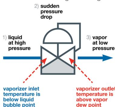
Figure 1. The three-stage vaporization process.
