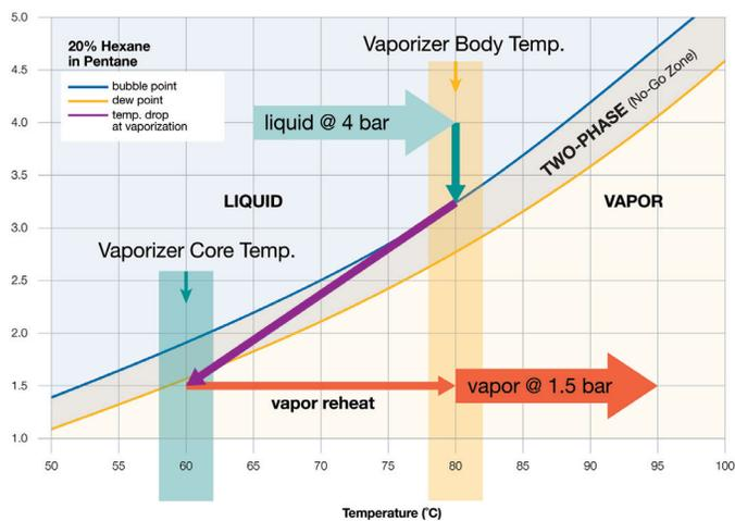
**Figure 2.** Phase diagram showing 20 percent hexane in pentane, with temperature settings
