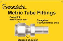
Note: These metric fittings are to be used on metric tubing sizes only. They are similar in appearance to Swagelok tube fittings in fractional sizes. The significant difference, however, is in the internal diameter of the tube fitting components. Due to the external similarity between metric and fractional sizes, a stepped shoulder is machined into the body and nut hex for easy identification. Shaped fittings are stamped MM.
