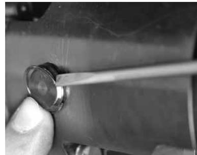
Fig. 20 Removing Clips from Retainer Shaft
