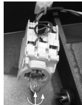
Fig. 27 Push and twist bulb CCW to remove.
