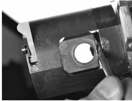
*Fig. 22 Applying Lubricant to Connector Shaft*
