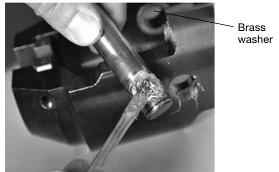
Fig. 21 Applying Lubricant to Retainer Shaft
