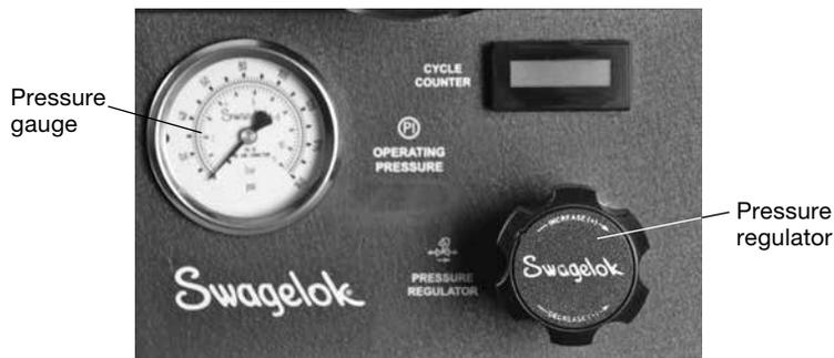
Fig. 12 Front Panel of HVSU
