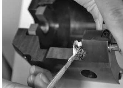
*Fig. 23 Applying Lubricant to Latch Pins*
