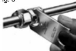
Position the Swagelok gap inspection gauge next to the gap between the nut and body. *Fig. 9.*
