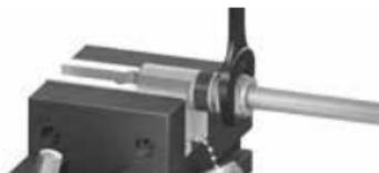
4. Loosen the nut and remove the tube with preswaged ferrules from the preswaging tool. If the tube sticks, gently rock it back and forth. Do not turn the tube. *Fig. 4*
