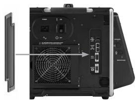
3. Install the new screws and tighten until screws and port cover are flush. Turn screws 1/16 turn past flush. Note: If the cover plate is removed, reinstall the screws on the power supply.
