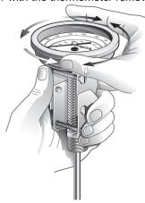
Rotate case/stem assembly to the desired position. Tighten both long screws.
