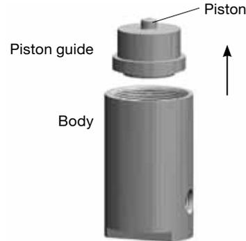
6. Lightly grip the **piston guide** in the vise and loosen the self-vent seat retainer from the piston guide using the **piston assembly bar** and **vent retainer tool**. The piston assembly bar must be held still.
