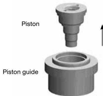
9. Remove the **piston seal** and the **backup ring** from the **piston guide**, and the **body seal** from the **body**.
