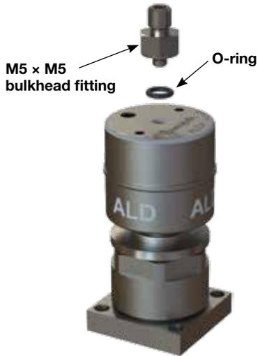
1. Install the **O-ring** into the groove of the **M5 x M5 bulkhead fitting**. Assemble the **M5 x M5 bulkhead fitting** assembly to the actuator cap and tighten between 5 to 15 in.-lb (0.5 to 1.6 N·m).
